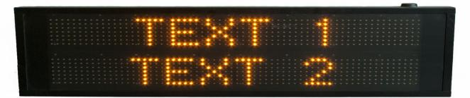
Matrix display, resolution(VxH): 7x64 pixels, pixel pitch 20 mm, Yellow LED field (VxH): 140x1280 mm Housing dimension (VxH): 450x1500mm (Two Line)
